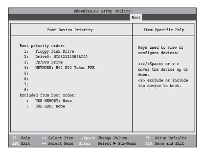
Figure 16. Boot Device Priority Submenu
